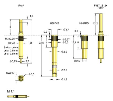
The probe F487 allows an exact determination of depths and lengths with low efforts. It was specifically developed for position tests at limited space. Due to the off-on-off function of the probe, the correct position of the DUT, a correct pin length or hole depth can be verified. The probe can be used with the standard receptacle H887RD or H887KB which allows a solderless exchange of the probes.
